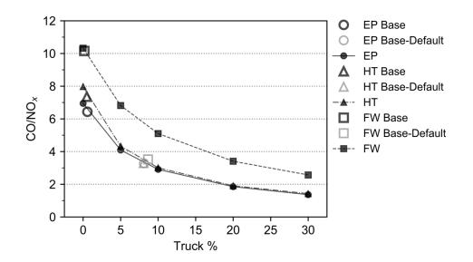
Figure 8. Annual morning peak time  $CO/NO_x$  ratios for fleet mix scenarios by fleet average truck percentage. Solid markers indicate the results for each sensitivity run using BAL data inputs for all other parameters examined.
