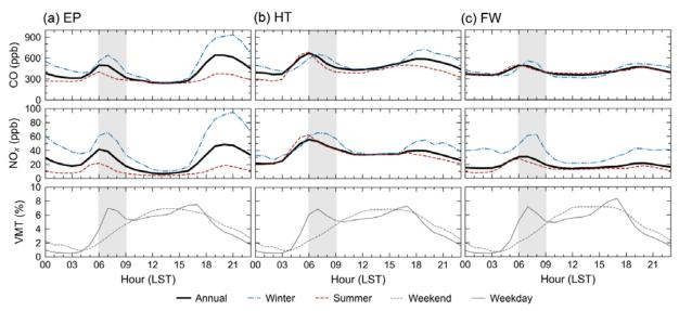
Figure 2. Mean diurnal profile of ambient hourly CO and NO<sub>x</sub> and hourly VMT distributions (percentage of passenger cars on urban freeways). VMT data were provided by TCEQ. Shaded background from 06:00 LST to 09:00 LST indicates the range of data used in subsequent analyses in this study.
