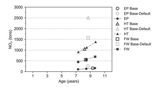
Figure 11. Annual morning peak time  $NO_x$  emissions for vehicle age scenarios by fleet average age. Solid markers indicate the results for each sensitivity run using BAL data inputs for all other parameters examined.
