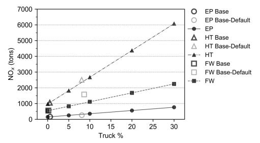
Figure 7. Annual morning peak time  $NO_x$  emissions for fleet mix scenarios by fleet average truck percentage. Solid markers indicate the results for each sensitivity run using BAL data inputs for all other parameters examined.
