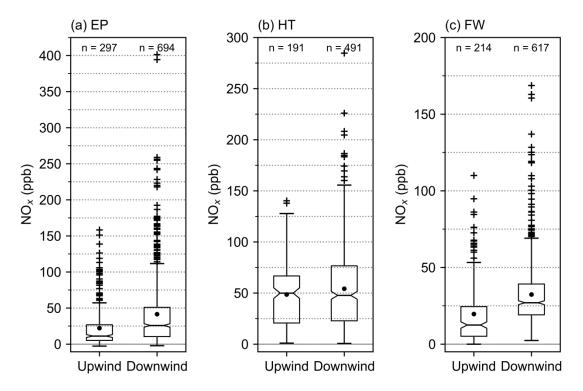
Figure 4. Distribution of  $NO_x$  mixing ratios from 06:00 LST to 09:00 LST when the monitor was located upwind and downwind of the target road. Outliers are indicated by crosshairs; the mean  $NO_x$  mixing ratio is represented by a black circle. The number of observations (n) used to compute the ambient statistics is shown above each data set.
