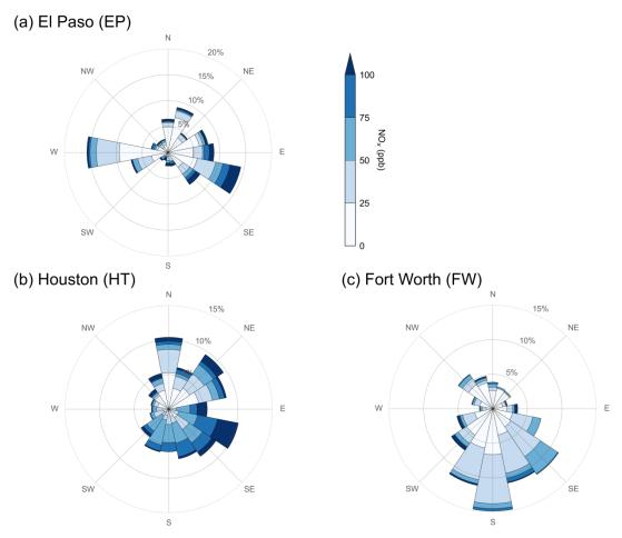
Figure 3. Distribution of NO<sub>x</sub> mixing ratios as a function of wind direction for morning hours (06:00 LST to 09:00 LST) in 2015 as a pollution rose. The wind direction is represented as the angular component, the percentage of data records is represented by the radial component, and NO<sub>x</sub> mixing ratios are represented by the color scale shown in the upper right.
