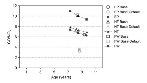
Figure 12. Annual morning peak time CO/NO<sub>x</sub> ratios for vehicle age scenarios by fleet average age. Solid markers indicate the results for each sensitivity run using BAL data inputs for all other parameters examined.
