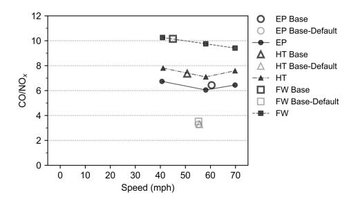
Figure 10. Annual morning peak time  $CO/NO_x$  ratios for vehicle speed scenarios by fleet average speed. Solid markers indicate the results for each sensitivity run using BAL data inputs for all other parameters examined.
