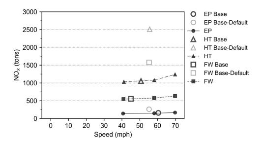
Figure 9. Annual morning peak time  $NO_x$  emissions for vehicle speed scenarios by fleet average speed. Solid markers indicate the results for each sensitivity run using BAL data inputs for all other parameters examined.
